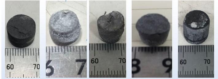
Before Sintering After sintering (No replacement) After sintering (10% TiC particle replacement) After sintering (15% TiC particle replacement) After sintering (20% TiC particle replacement)
