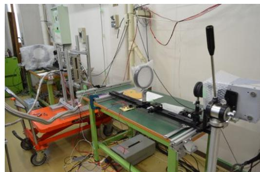
Figure 5: Experimental setup of schlieren optical measurement system
